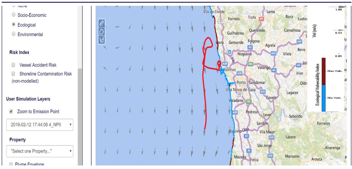
**Fig. 1.** Pre-spill area and spill occurrence (72 h) (top to bottom). The red circle bullet represents the spill emission point and the red solid line the plume centre trajectory during the 3 d of simulation. The ecological vulnerability index is represented in a contour along the shoreline, grey arrows represent the current velocity (m/s). (For interpretation of the references to colour in this figure legend, the reader is referred to the web version of this article.)
