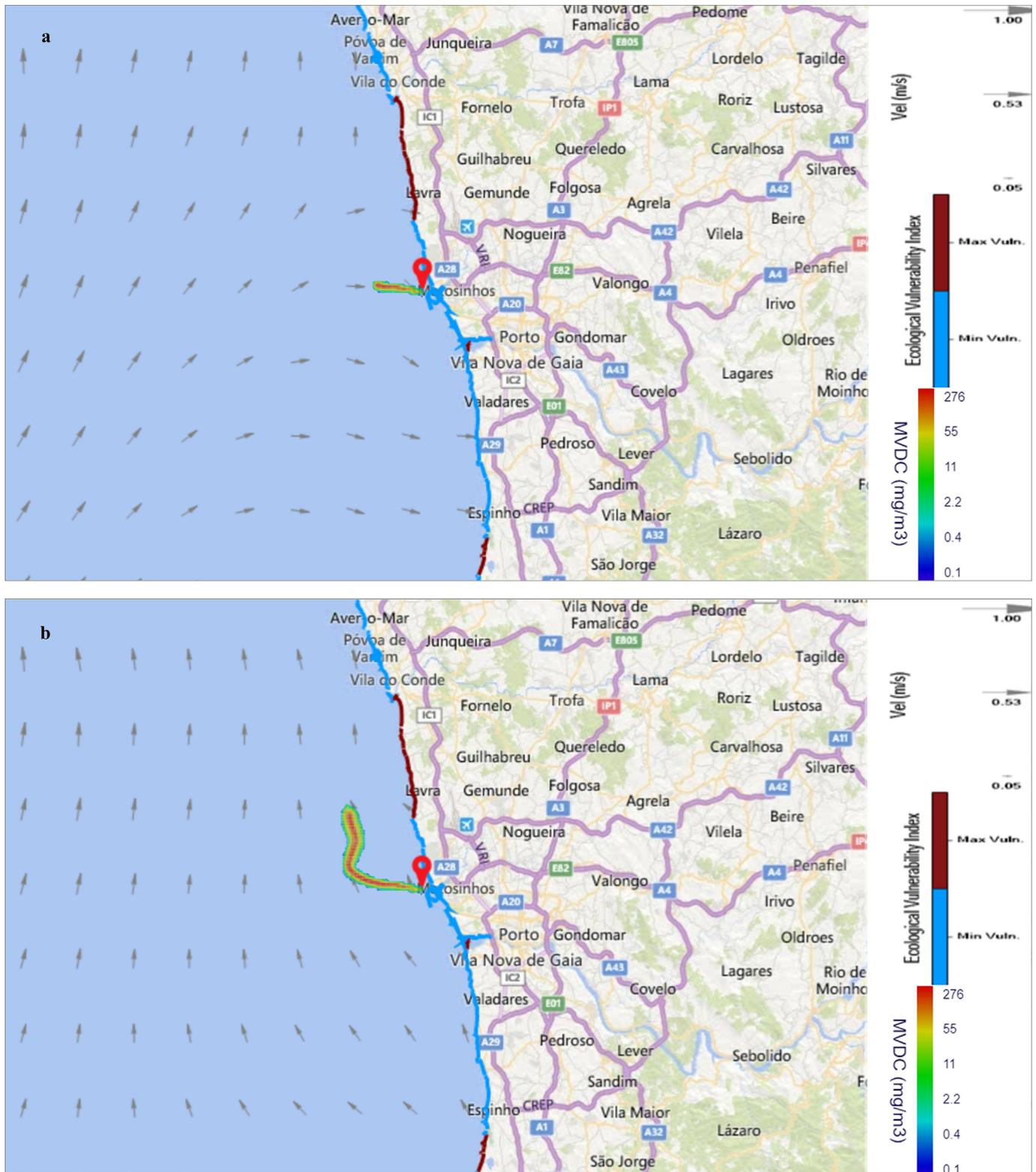
**Fig. 2.** Maximum time-integrated vertical dissolved concentration (MVDC, mg/m<sup>3</sup>) after 6 (a), 24 (b), 48 (c) and 72 h (d) post 4-NP spill simulation. The red circle bullet represents the spill emission point and grey arrows the current velocity (m/s). The ecological vulnerability index is represented in a contour along the shoreline. (For interpretation of the references to colour in this figure legend, the reader is referred to the web version of this article.)
