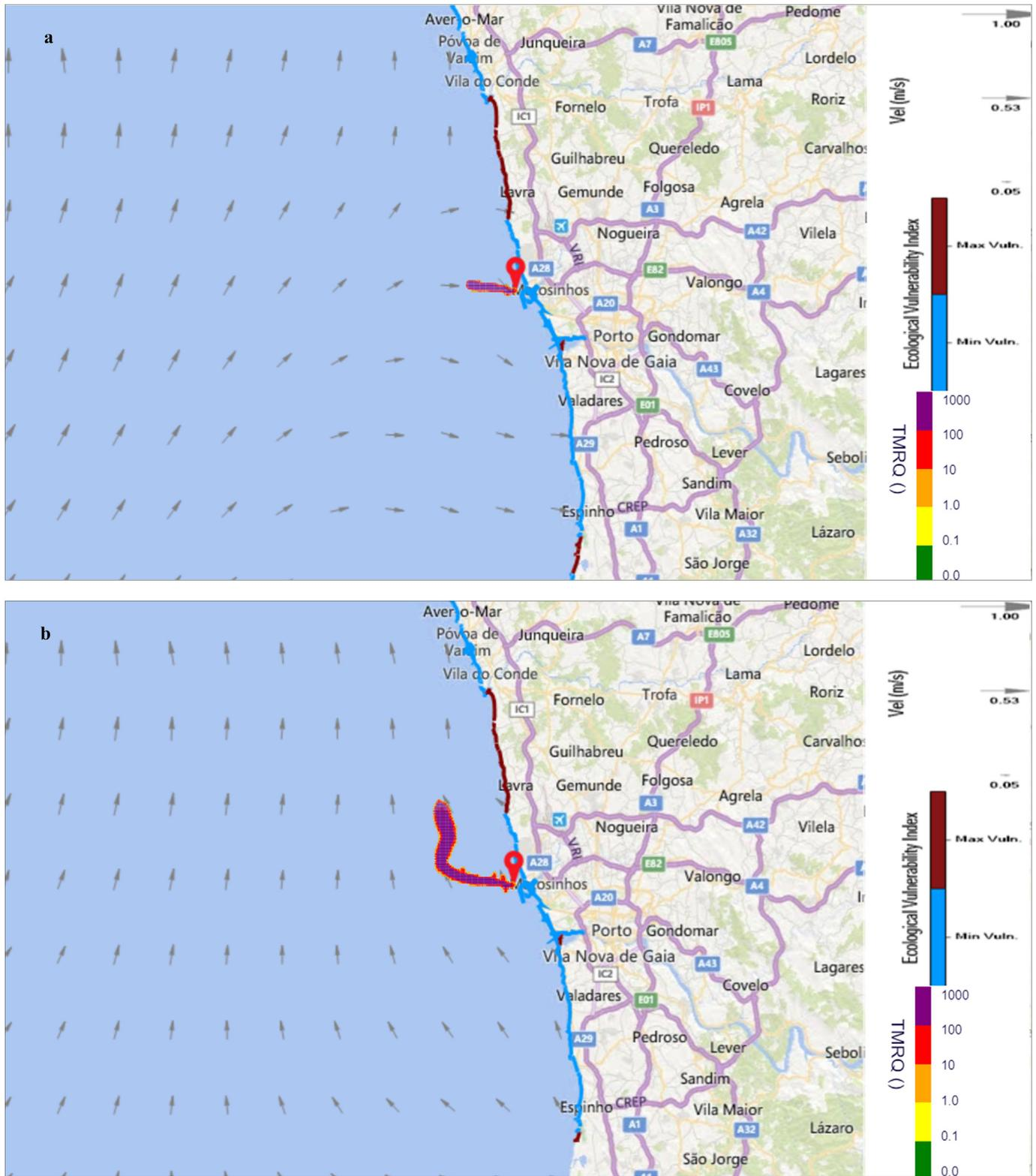
**Fig. 3.** Toxicity/maximum time-integrated Risk Quotient (TMRQ) after 6 (a), 24 (b), 48 (c) and 72 h (d) post 4-NP spill simulation. The red circle bullet represents the spill emission point and grey arrows the current velocity (m/s). The ecological vulnerability index is represented in a contour along the shoreline. (For interpretation of the references to colour in this figure legend, the reader is referred to the web version of this article.)
